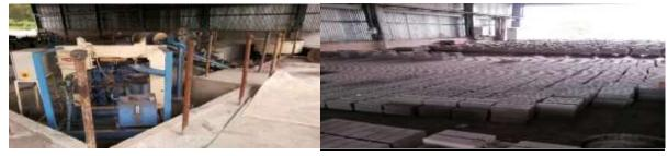
**Reduces air pollution** - Fossil fuel is used in heating clay bricks in kilns. Burning such fuel generates air pollution and greenhouse gas (CO2), contributing to global warming. Fly ash bricks are manufactured at room temperature and there is no fossil fuel burning and emission of green house gas (Co2).
