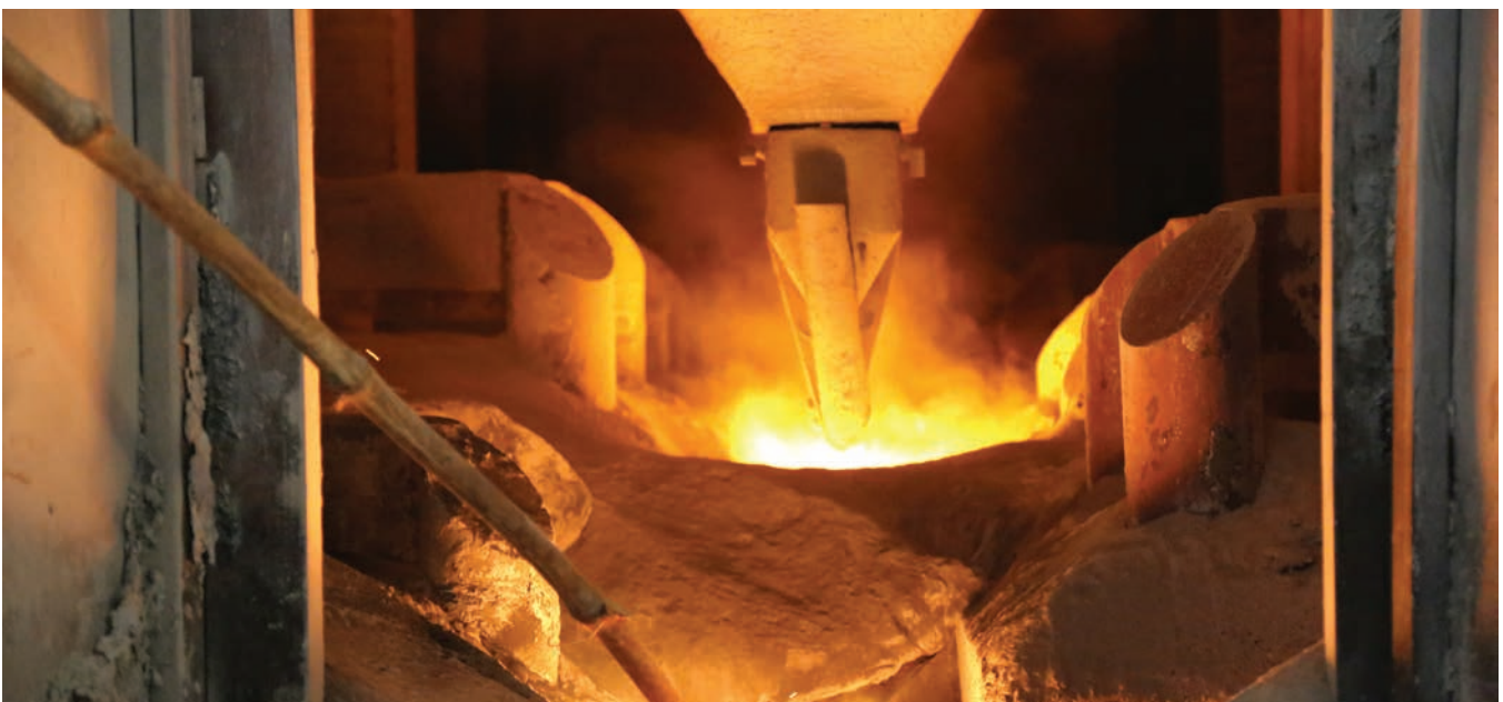
Inside view of electrolytic pot at Aluminium Smelter
