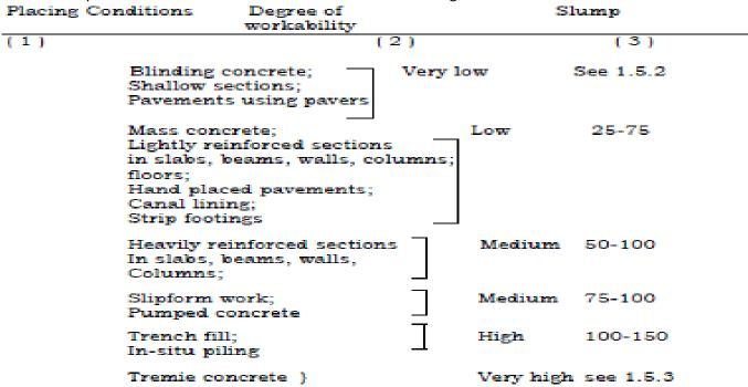
Note: For most of the placing conditions, internal vibrators (needle vibrators) are suitable. The diameter of the needle shall be determined based on the density and spacing of reinforcement bars and thickness of sections. For tremie concrete, vibrators are not required to be used.
