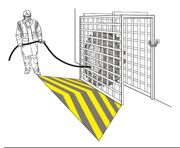
A strong, firmly-secured cage. Consider lining this with mesh to retain debris. For fixed installations it is helpful to mark the safety exclusion zone
