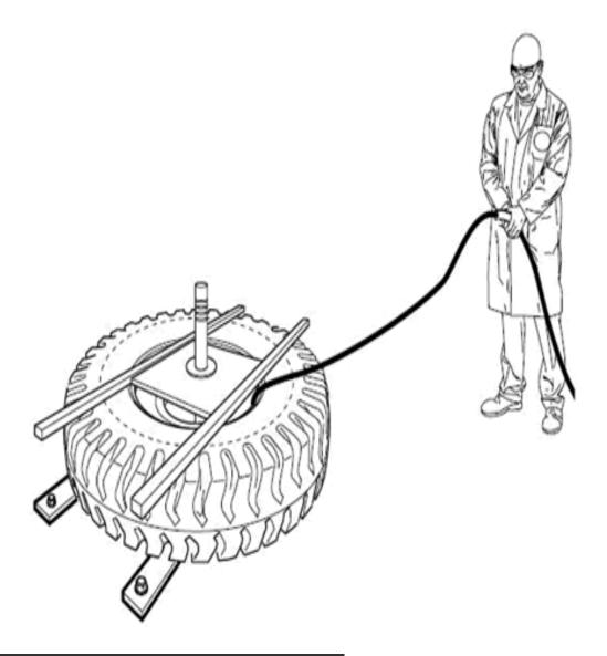
A secured horizontal stool and associated clamping mechanism
