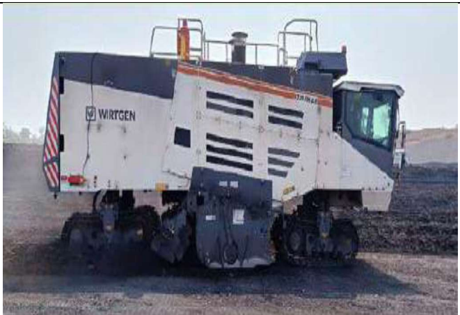
Surface Miner with water spray
